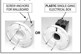
Step 7. Attach the GEM-SMK-1 to mounting plate.
