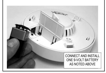
The smoke alarm and transmitter are powered by one 9-volt alkaline battery (supplied) which can power the unit for at least one year. If the battery voltage drops below normal, a low-battery report will be sent to the receiver with any status or alarm transmission. If a low-battery condition is indicated, replace battery.
