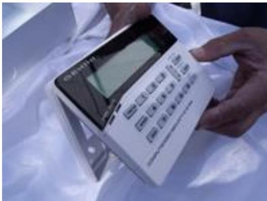
4. Mount keypad base with small sheet rock screws. Drill large hole near bottom of large rectangular hole in base plate to allow connection of wire harness.
