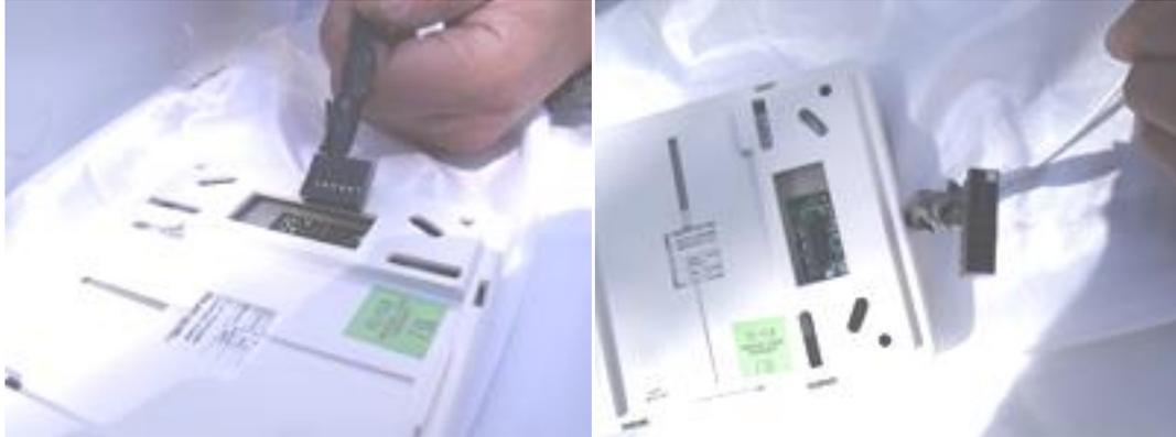
6. Hook keypad on top hinges of base plate. While pushing down on keypad, snap both bottom clasps.
