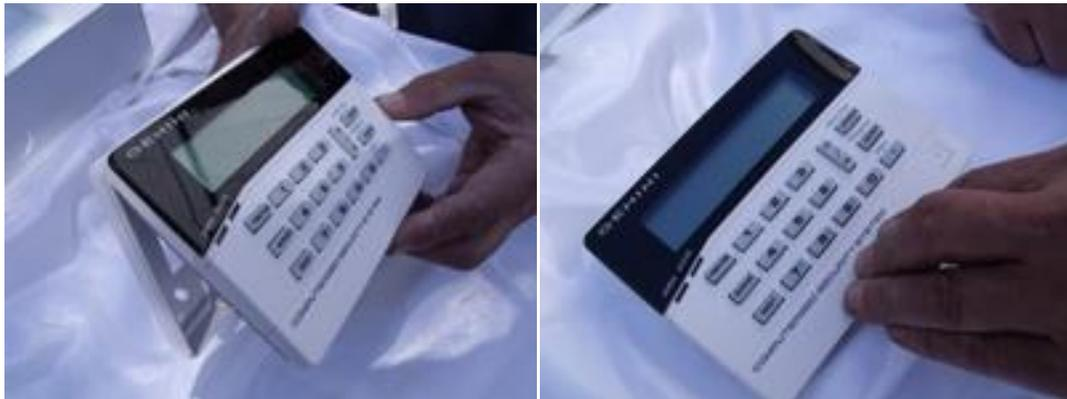
7. Run wire from keypad to control panel enclosure thru top grommet. You may cut off any excess wire and restripe ends. Connect wires by color codes in picture.
